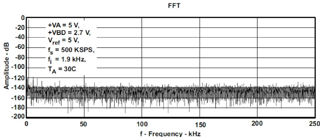
**Figure 6. Typical ADC Output Spectrum Plot**
