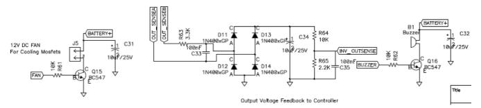
Figure 16. Output Sense, DC Fan, and Buzzer Operations
