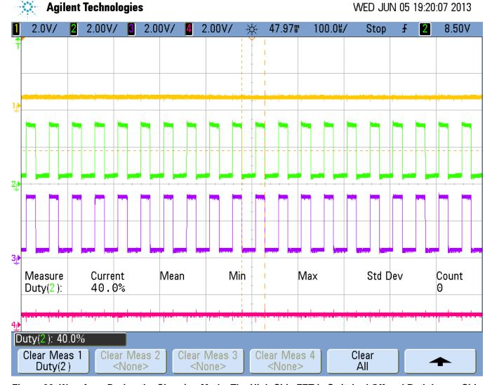
Figure 30. Waveform During the Charging Mode. The High-Side FET is Switched Off and Both Lower-Side FETs to Ground in the H Bridge are Switched at the Same Time With the Duty Cycle Proportional to the Battery Charge Current
