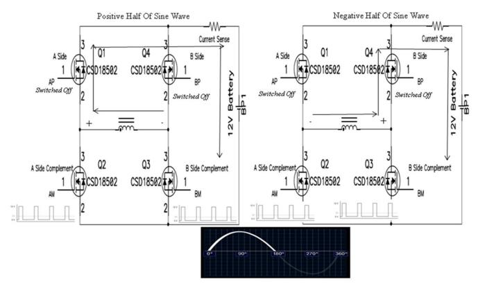
Figure 8. Charging Mode PWM Switching Explanation
