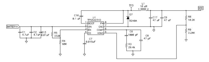
3.3V Output from DC/DC Converter
