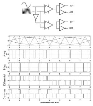
Figure 6. Waveform Generation in Inverter Mode
