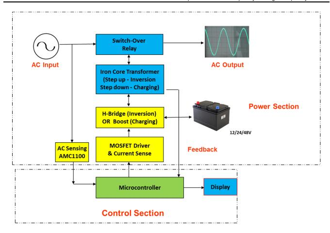
Figure 31. Bidirectional Low Frequency Inverter
