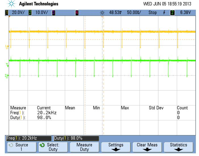
Figure 27. Maximum Duty Cycle of the PWM Switching at 400 W (at the Inverter's Output) is Increased to 98 Percent to Maintain Voltage regulation at the Inverter's Output by Sensing the Auxiliary Winding. This Results in Slight clipping of Sinusoidal Waveform at theOutput.
