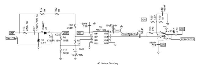
Figure 14. AC Mains Sensing Through Isolated Amplifier
