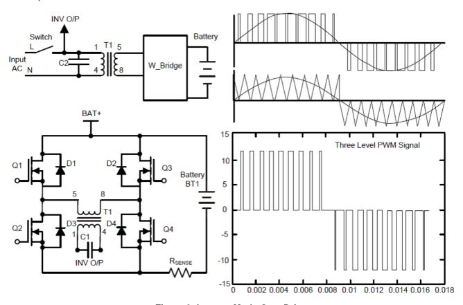
Figure 3. Inverter Mode Gate Drives
