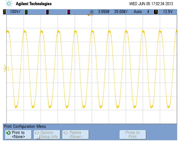
Figure 29. Inverter's Output at 400-W Load With 12-V Battery Input
