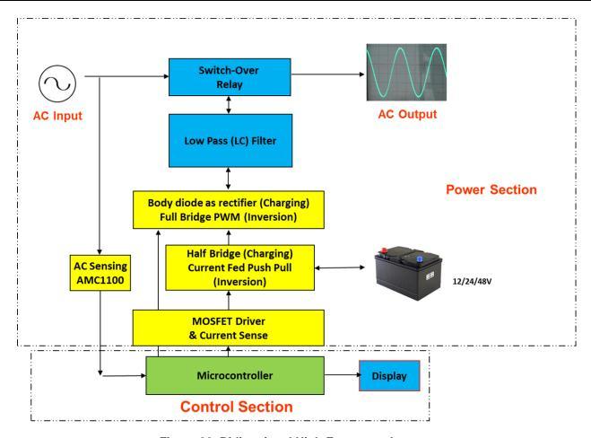
Figure 32. Bidirectional High-Frequency Inverter
