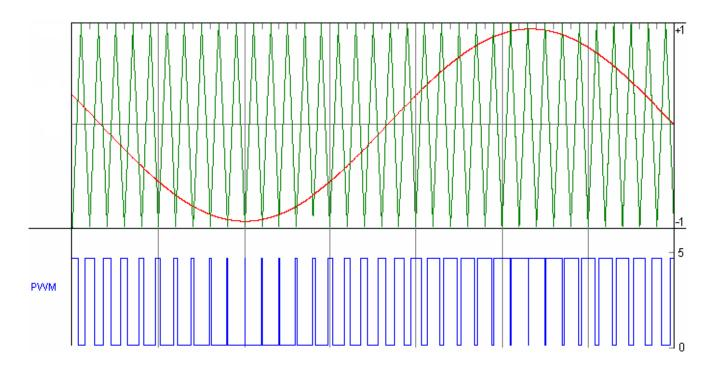
Figure 5. Modulation of Sine Wave With Higher Frequency PWM Signals
