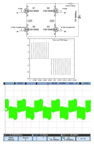
Figure 22. Trilevel Switching Across the High-Side A MOSFETS Source (HSA) and High-Side B MOSFETs Source (HSB).
