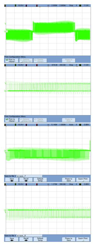
Figure 23. Trilevel Switching Across the High-Side A MOSFETS Source (HSA) and High-Side B MOSFETs Source (HSB).
