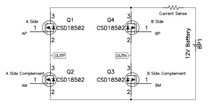
Figure 4. H Bridge Configuration of MOSFETs
