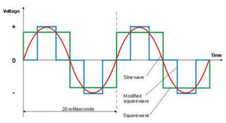
Figure 1. Types of Inverter Outputs
