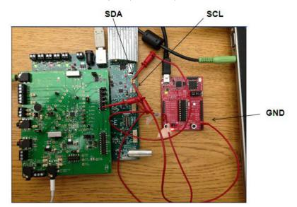
**Figure 4. Hardware Connection**
