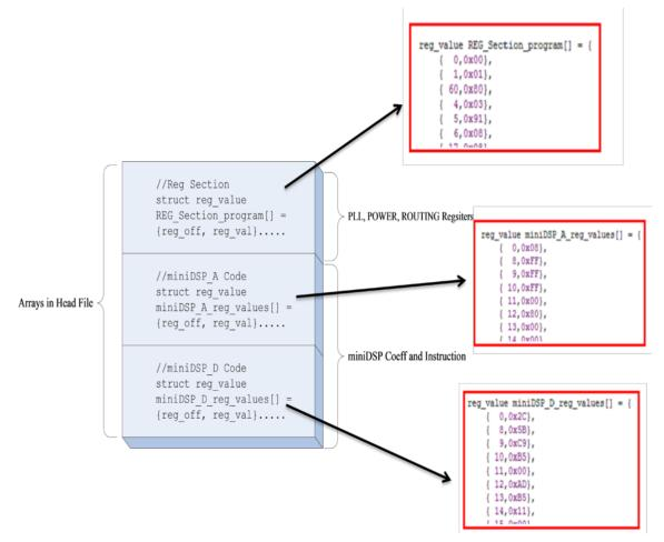
Figure 13. miniDSP Head File Structure
