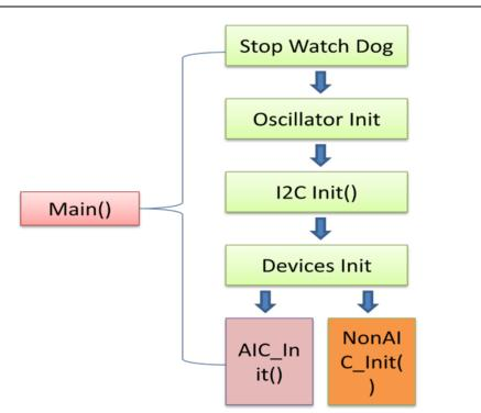
Figure 2. Main.c File Function Flow
