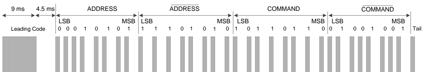
Figure 13. Pulse Distance Protocol, Data Frame Format
