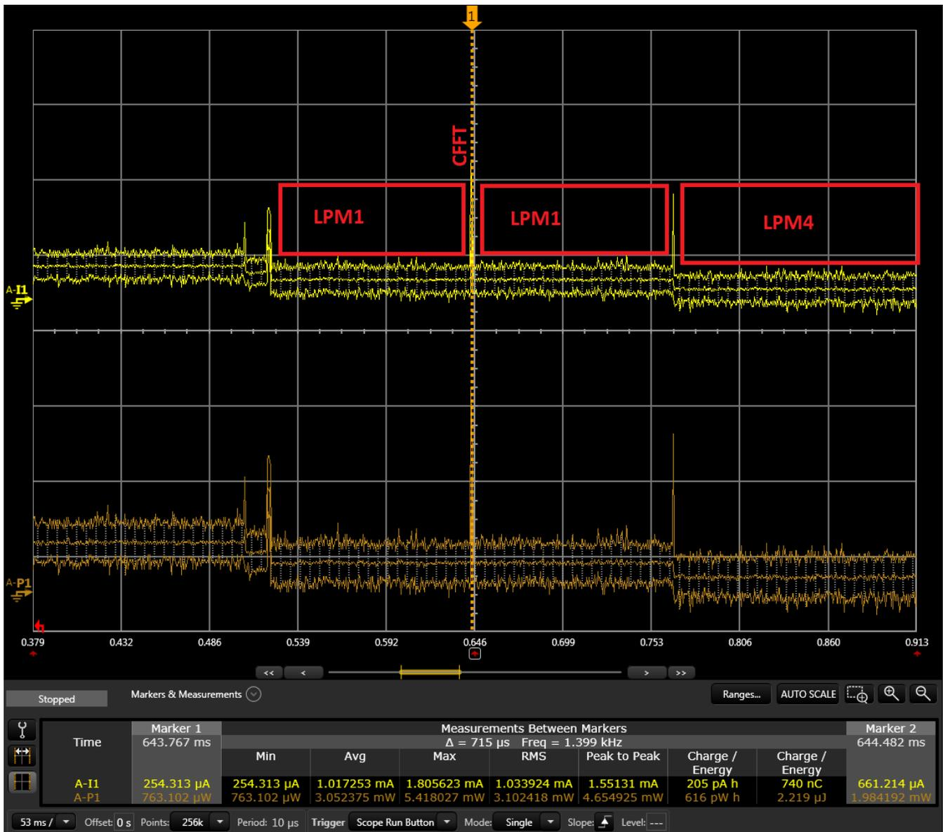
Figure 11. 256-Point Complex FFT With the LEA Module Enabled
