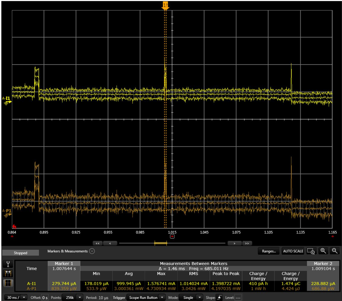
Figure 12. 512-Point Complex FFT Running at 8 MHz With the LEA Module Enabled
