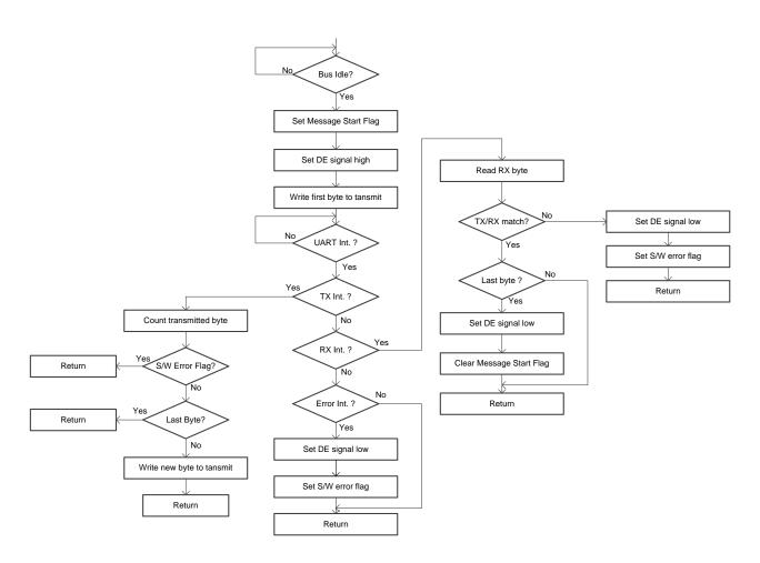
Figure 2. Process of Sending a RS-485 Message
