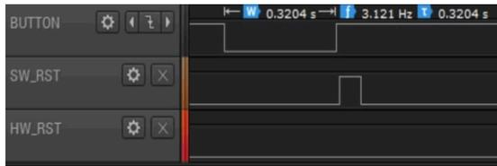
**Figure 2. Soft Reset Pulse (SW\_RST)**
