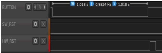
**Figure 3. Hard Reset Pulse (HW\_RST)**
