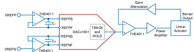
Figure 2. DACx1001 Control Loop Schematic
