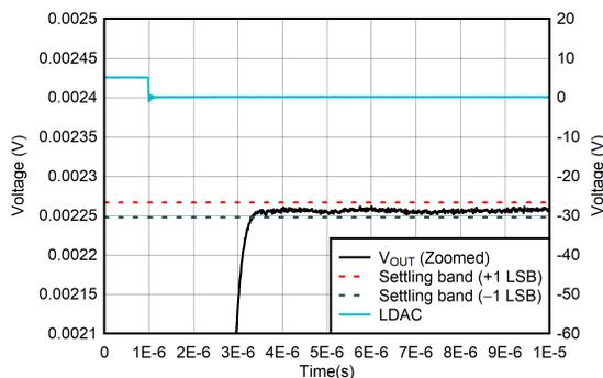
**Figure 4. DAC11001A Output Settling**
