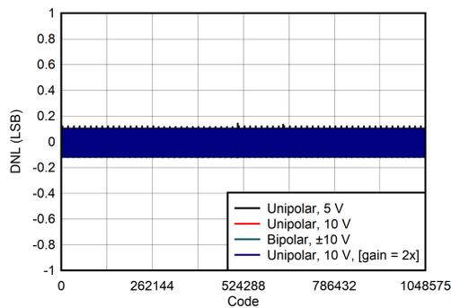
**Figure 3. DAC11001A DNL versus Digital Code**
