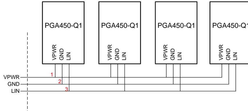
**Figure 1. 3-Wire Connection**
