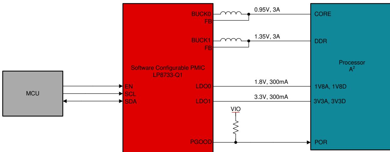
**Figure 6. Higher Current PMIC Processor Power**
