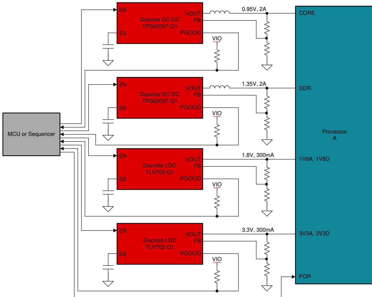
**Figure 1. Discrete Processor Power**
