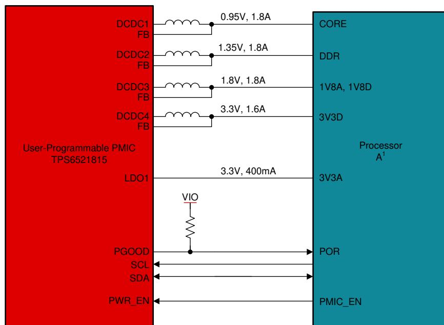
**Figure 7. User-Programmable PMIC Processor Power**
