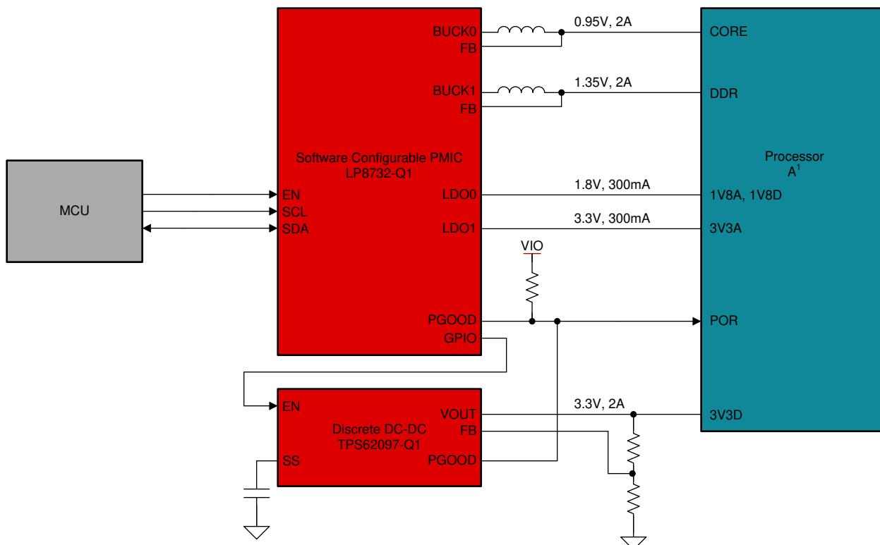
**Figure 4. Hybrid (PMIC plus Discrete) Processor Power**
