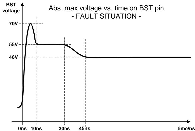
Figure 2 Absolute Maximum Voltage vs. Time, Rising Edge Transition on BST, Fault Situation
