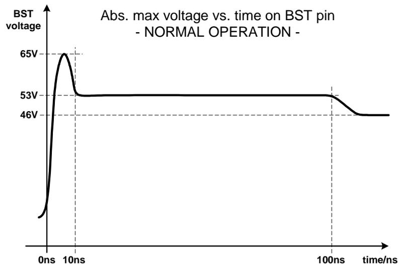
**Figure 1 Absolute Maximum Voltage vs. Time, Rising Edge Transition on BST, Normal Operation**
