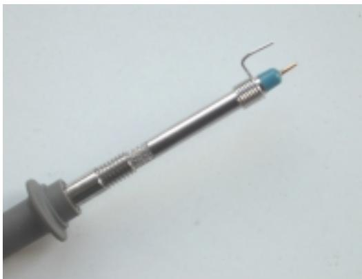
**Figure 3 This is how the ground wire should look**
