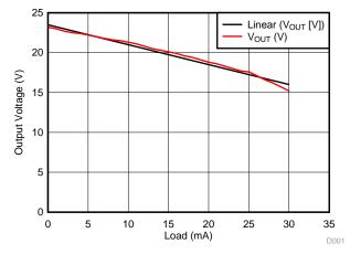
Figure 5. Charge-Pump Output Voltage versus Load Current
