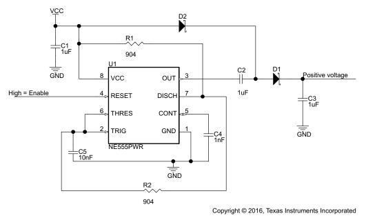
Figure 2. Positive Charge-Pump Circuit
