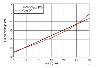
Figure 9. Charge Pump Output Voltage versus Load Current
