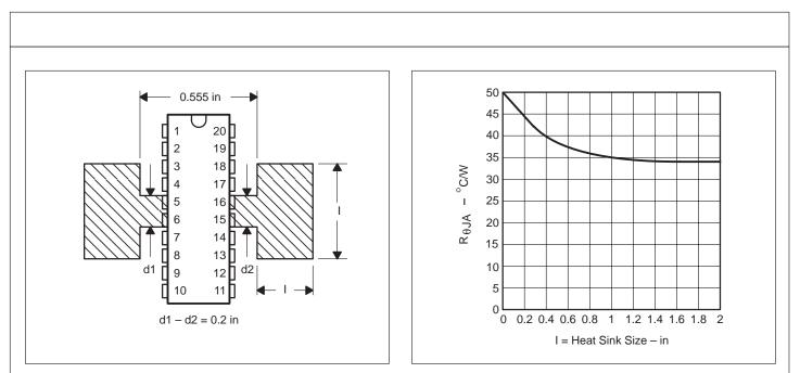
Figure 7. Copper PC Board Used as a Heat Sink
