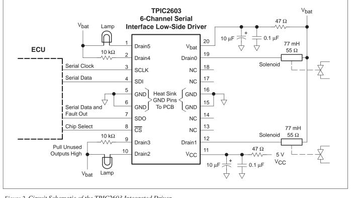
Figure 2. Circuit Schematic of the TPIC2603 Integrated Driver
