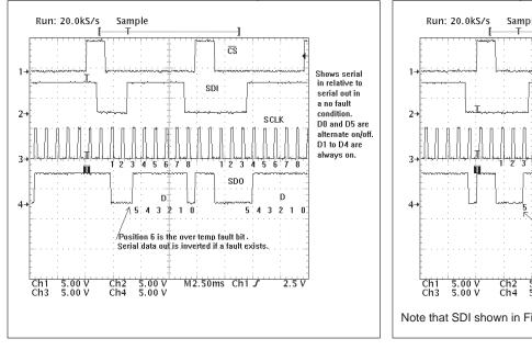
Figure 3. Serial Data Transfer
