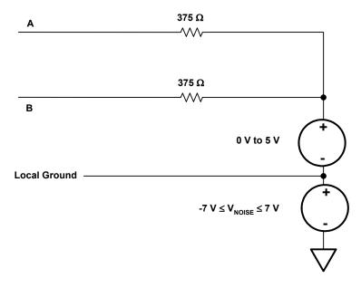
Figure 5. Physical Representation of the Test Circuit
