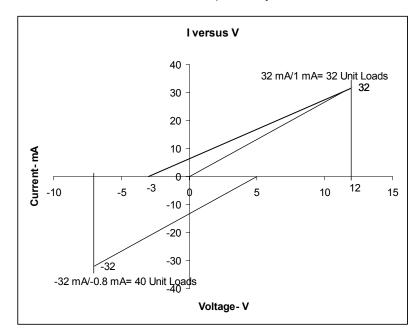
Figure 6. Unit Loading of Common-Mode Test Circuit
