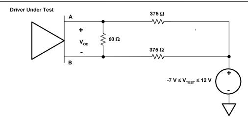
Figure 4. Differential Output Voltages With Common-Mode Loading
