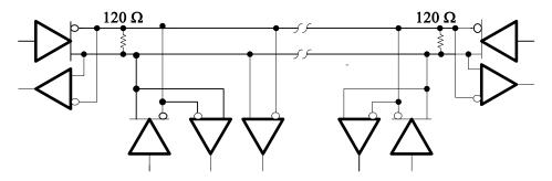
Figure 1. Example Schematic of a Multipoint Bus
