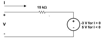
Figure 2. Electrical Model of One Unit Load
