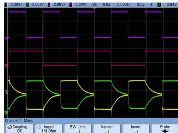
Transmitter test w/o dump resistor.
