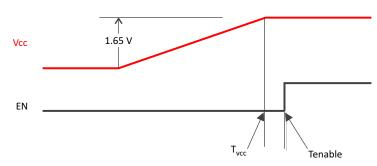
Figure 2. Cold Start Vcc Ramp Up to EN
