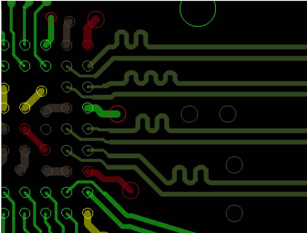
**Figure 4. DisplayPort Main Link Routing Example**
