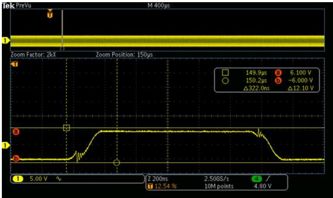
Switching Waveform on D1 at 200 mA Load for -6818 Transformer
