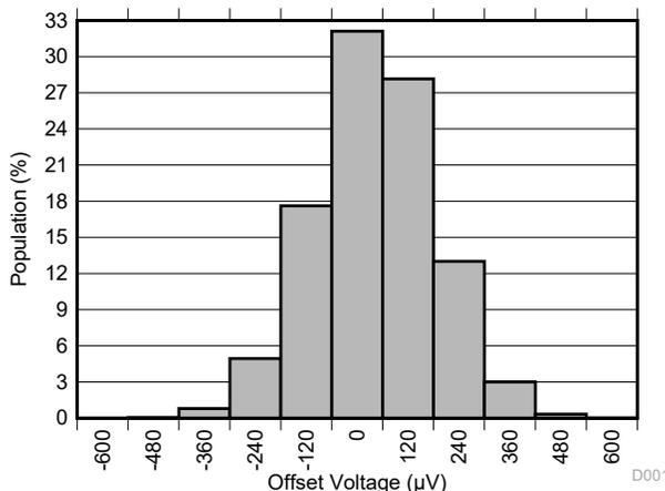
Figure 2-1. Distribution of  $V_{OS}$  for the OPA2991
