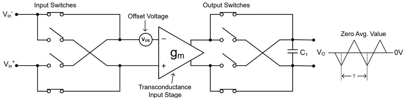
Figure 6-5. Chopper-Stabilized Amplifier
