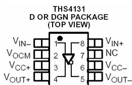
Figure 13. Pin Number Assignments for the THS 4131
