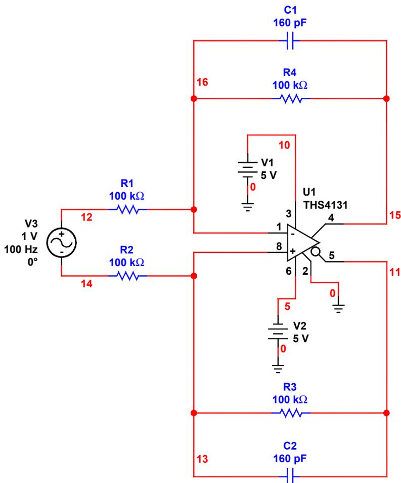
Figure 20. Electronics Workbench Schematic, Using New Symbol
