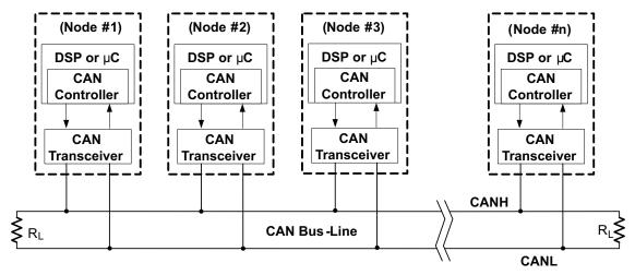
Figure 6. Details of a CAN Bus
