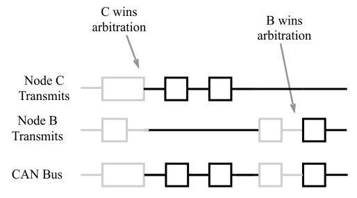
Figure 5. Arbitration on a CAN Bus
