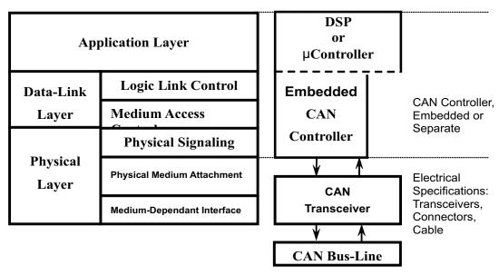
Figure 1. The Layered ISO 11898 Standard Architecture
