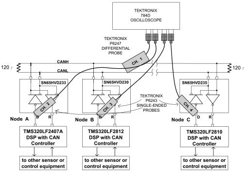
Figure 9. CAN Test Bus
