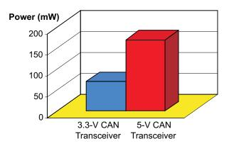
Figure 10. 3.3-V CAN Transceiver Power Savings
