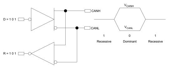
Figure 4. The Inverted Logic of a CAN Bus
