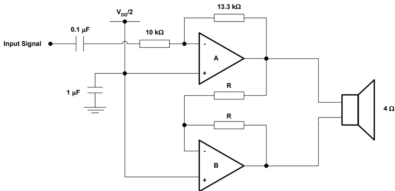
**Figure 4. The BTL Audio Power Amplifier Example**
