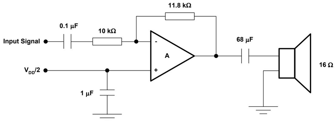
**Figure 2. The SE Audio Power Amplifier Example**
