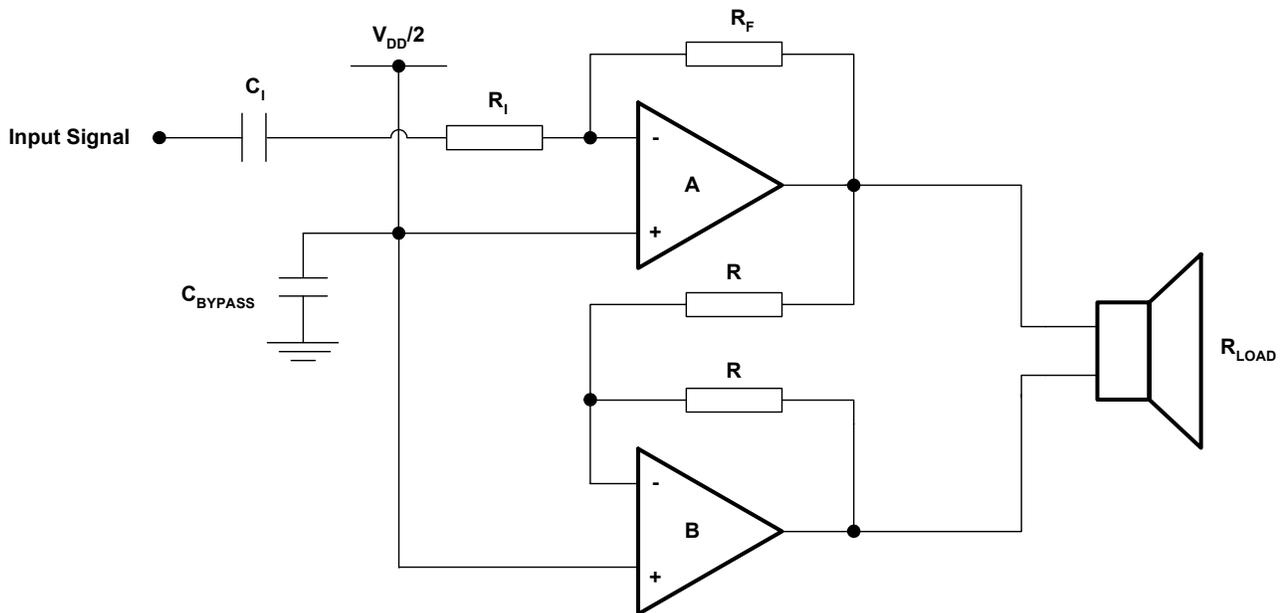
**Figure 3. The BTL Audio Power Amplifier**
