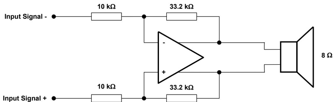
Figure 7. The Fully Differential Audio Power Amplifier Example
