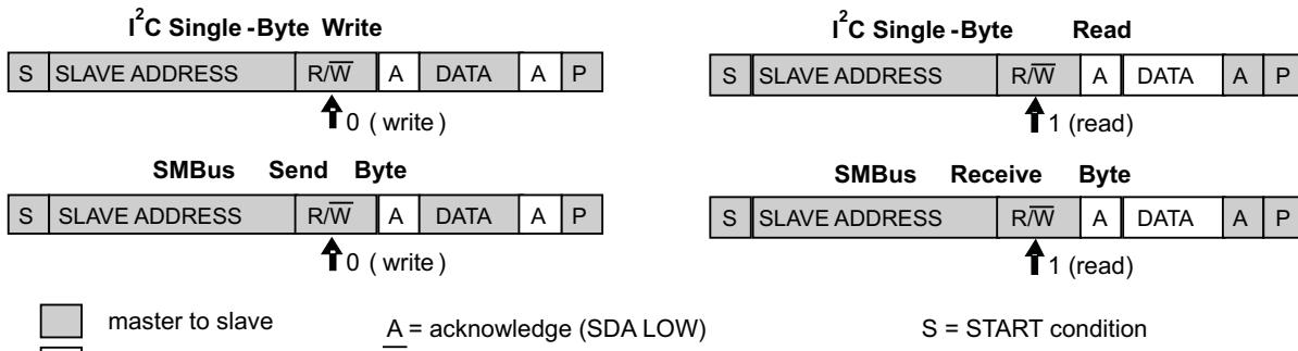
**Figure 1. I<sup>2</sup>C Single-Byte Write and Read Compared to SMBus Send and Receive Byte**
