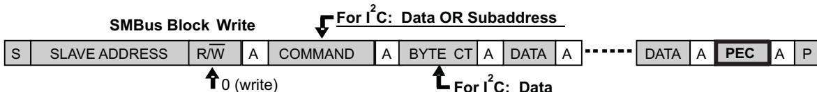
**Figure 4. SMBus Packet Error Checking (PEC)**
