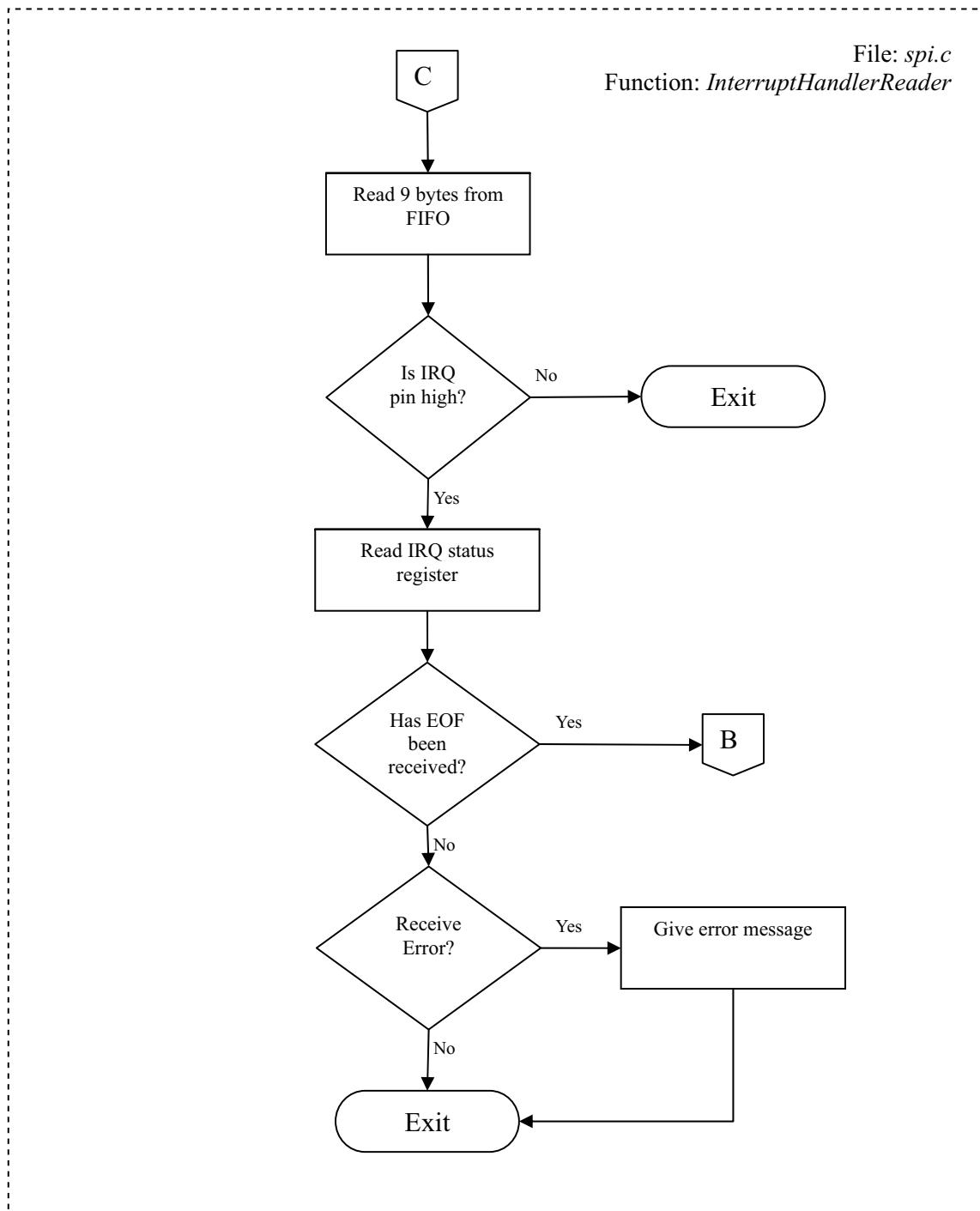
Figure 4. Inerrupt Handler Routine (3)
