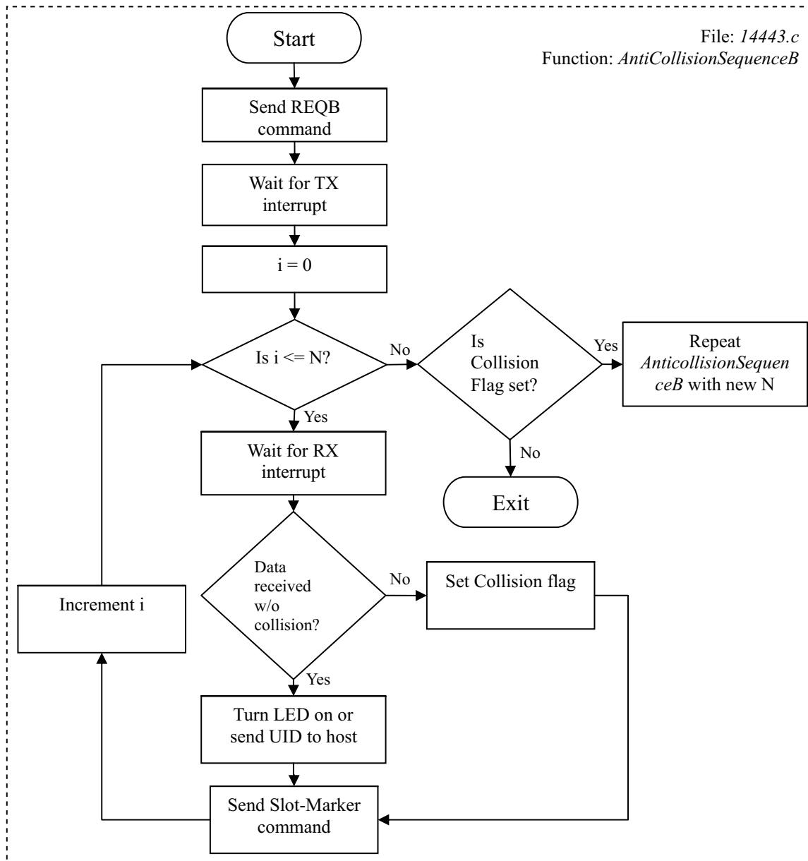
**Figure 1. AntiCollisionLoop**
