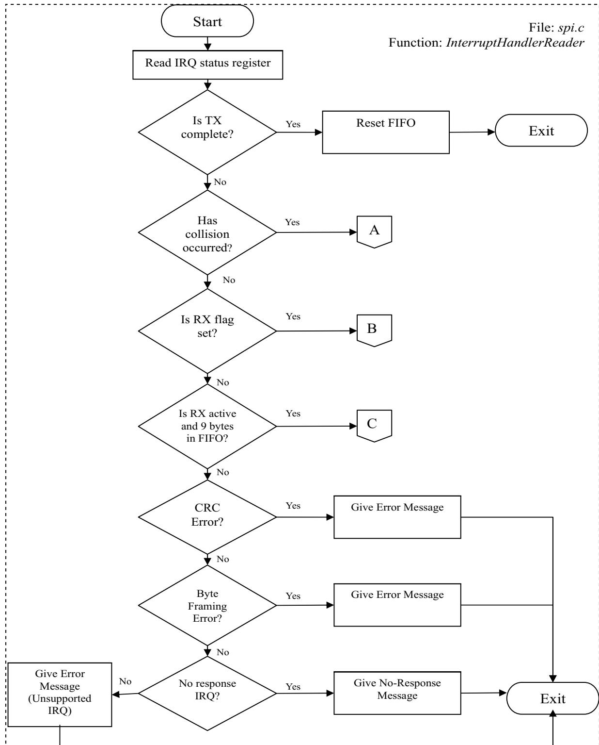
**Figure 2. Inerrupt Handler Routine (1)**
