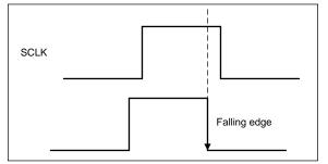
Communication is terminated by the parallel mode Stop condition when MOSI data changes during a high SCLK period.
