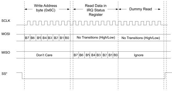
Figure 4. SPI Interface Communication (IRQ Status Register Read)
