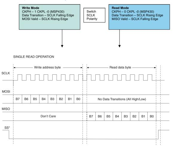
Figure 2. Serial - SPI Interface Communication (Read Mode)
