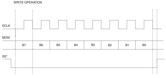
Figure 1. Serial - SPI Interface Communication (Write Mode)
