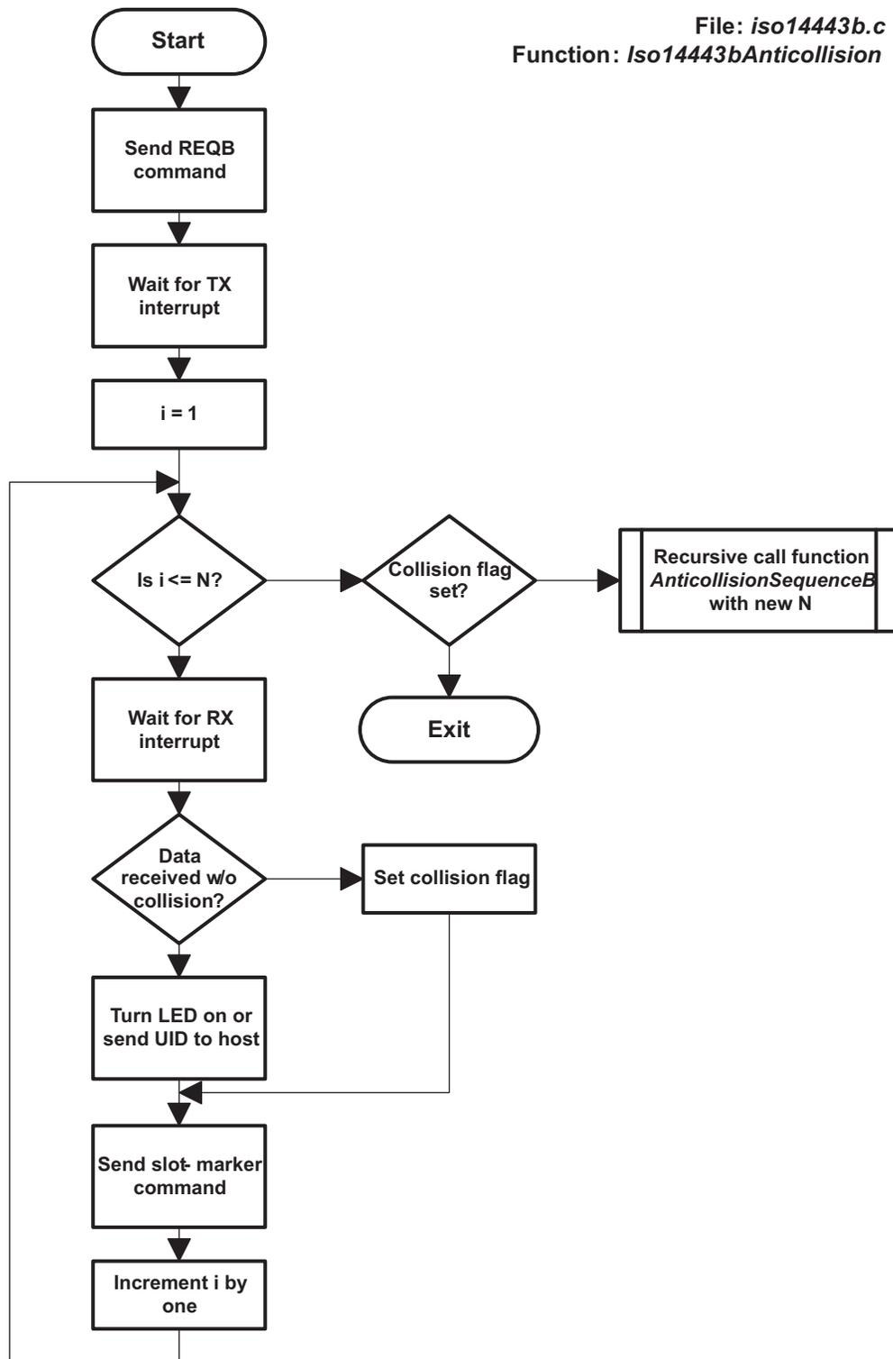
Figure 10. ISO14443B Anti-Collision Method Flow Chart
