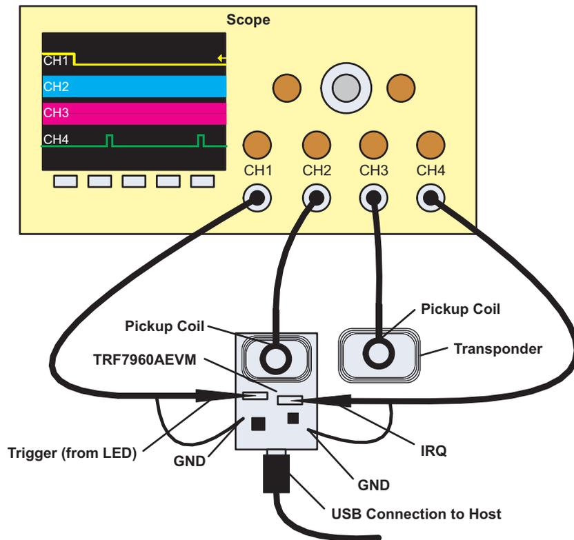
Figure 12. Measurement Setup for Using Trigger Feature
