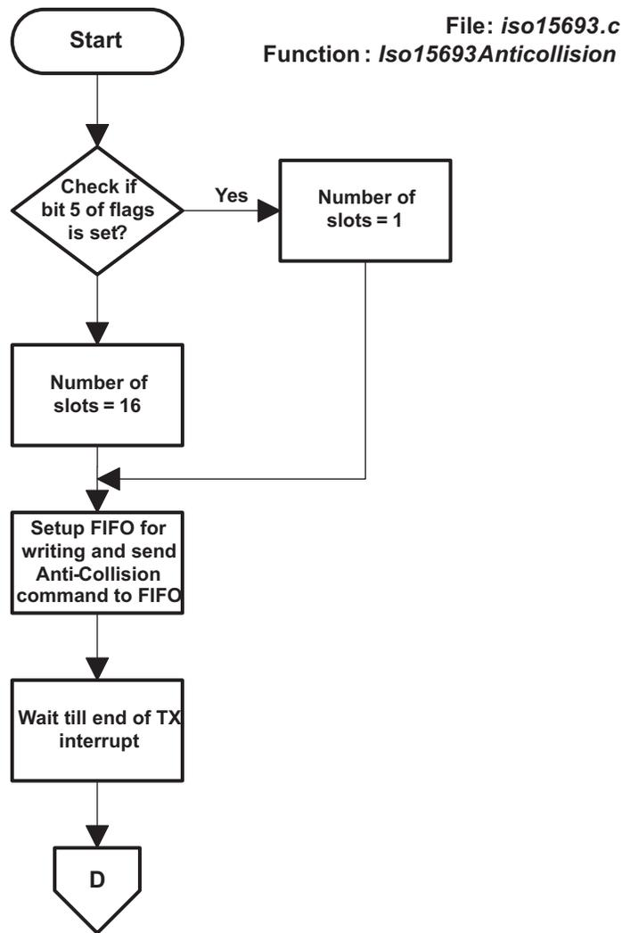
Figure 7. ISO15693 Anti-Collision Method Flow Chart (1)
