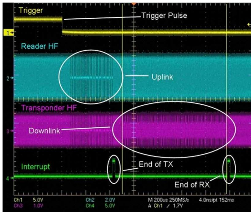
Figure 13. Oscilloscope Screen Example Using Trigger Feature
