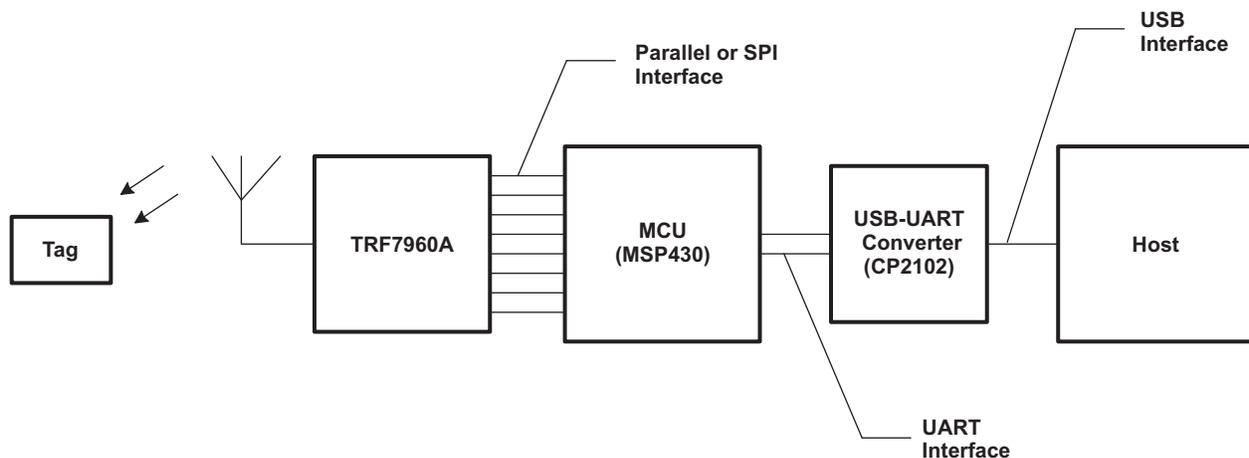
**Figure 1. TRF7960A EVM Application Block Diagram**
