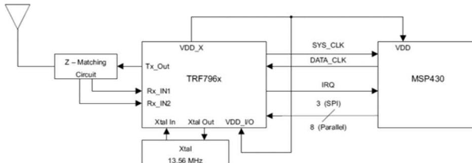
**Figure 2. TRF7960A Embedded System Block Diagram**
