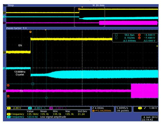
Figure 2. TX Out Behavior When EN is Line Raised (Register 0x0B set to 0x07)
