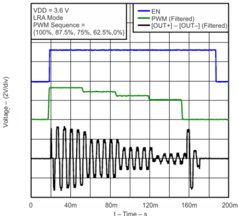
**Figure 1-1. LRA Auto-Resonance Detection**
