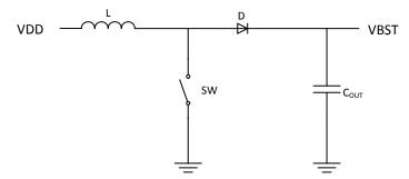
To convert the low voltage to a high voltage, the boost converter operates in two phases. In the first phase the inductor is charged by closing the switch and forcing current through the inductor to ground. During this period the current through the inductor increases allowing the inductor to store charge.
