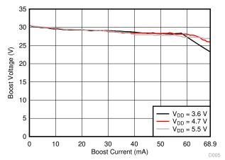
Figure 2-5. Load Regulation with  $V_{BST} = 30 \text{ V}$
