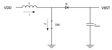
Once the inductor current reaches a maximum threshold, the switch opens and forces the inductor to dump the stored charge through the diode and onto the output capacitor and load.
