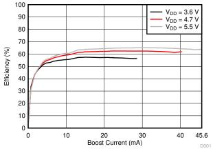
Figure 2-2. Efficiency with  $V_{BST} = 55 \text{ V}$
