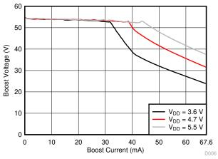
Figure 2-6. Load Regulation with  $V_{BST} = 55 \text{ V}$
