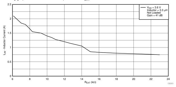
Use the R<sub>FXT</sub> resistor to set the current limit for the inductor. This can serve two purposes:
