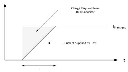
When a bulk input capacitor is included, the following diagram shows that the battery actually sees a filtered version of  $I_{I\,IM}$ .
