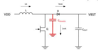
Both of these issues can have drastic effects on the output waveform. To identify switch node parasitic capacitance, look for continuous switching on the SW pin. During normal operation, the switching turns on and off depending on the current required; however, with parasitic capacitance the SW node often continuously switches to recover for lost switch cycles and current.
