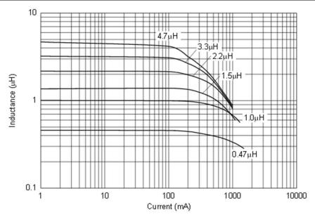
Figure 6-1. Inductance vs DC Current
