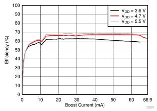
Figure 2-1. Efficiency with  $V_{BST} = 30 \text{ V}$
