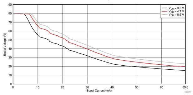
Figure 11-5. Boost Voltage vs Boost Current - DRV2667EVM-CT-80 V
