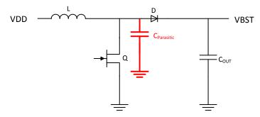
Figure 10-1. SW Node Parasitic Capacitance
