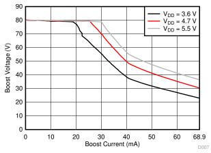
Figure 2-7. Load Regulation with  $V_{BST} = 80 \text{ V}$
