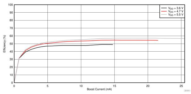
Figure 11-3. Boost Efficiency
