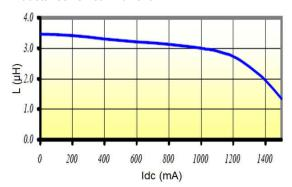
Inductor 1 (on the left) has a *Rated DC Current* of 1.2 A and Inductor 2 has a *Rated DC Current* between 1.1–1.3 A. Initially, both seem to work if our boost configuration requires 1 A; however, they are not equal.
