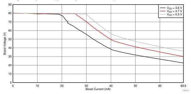
Figure 11-2. Actual Load Regulation and Boost Efficiency
