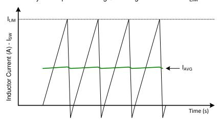
Calculating the exact  $I_{AVG}$  value is rather difficult, but as long as the bulk decoupling capacitance in the system is sufficiently high, the average current drawn from the battery will be less than one-half of  $I_{LIM}$  as a general guideline.
