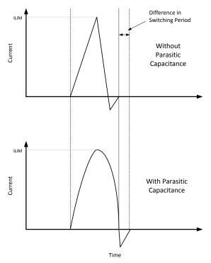
Figure 10-2. Inductor Charging with Parasitic Capacitance
