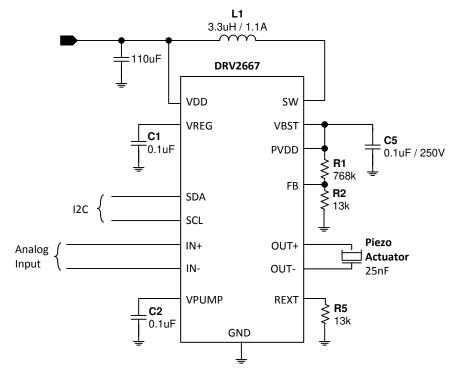
Figure 11-4. Simplified Version of the DRV2667EVM-CT Schematic
