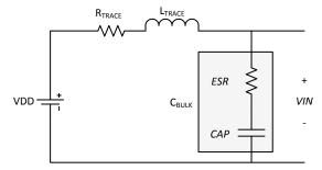
Keep in mind that it is difficult to calculate the exact input current required for the DRVxxxx, so a minimum capacitance between 22  $\mu$ F and 47  $\mu$ F is recommend.
