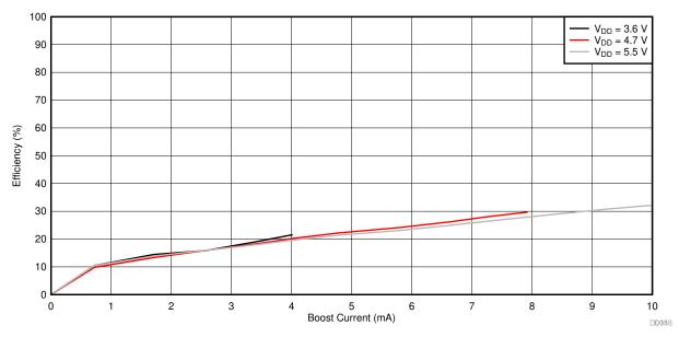
Figure 11-6. Efficiency vs Boost Current - V<sub>BST</sub> = 80 V
