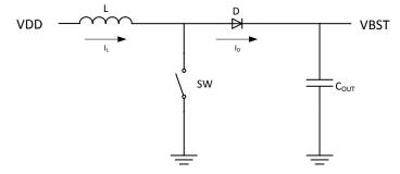
By repeating this charge and dump process, the boost converter is able to increase the output voltage.
