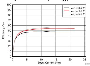
Figure 2-3. Efficiency with  $V_{BST} = 80 \text{ V}$
