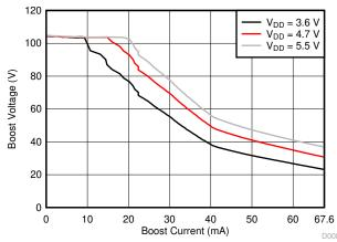
Figure 2-8. Load Regulation with V<sub>BST</sub> = 105 V
