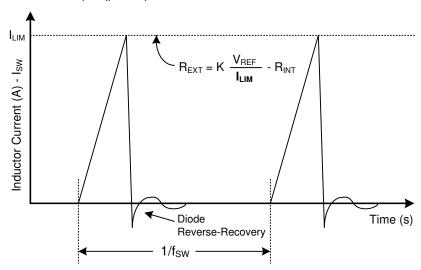
The boost converter only switches when the output voltage ( $V_{BST}$ ) is below the final target value, meaning that it will only switch when it needs to. Unlike a fixed-frequency boost converter design, the hysteretic boost converter design has a continually varying switching frequency and is load-dependent. Note that the DRV8662, DRV2665, and DRV2667 have forced switching at approximately 37 kHz.
