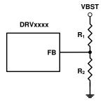
The boost feedback resistors can be calculated using equation Equation 2:
