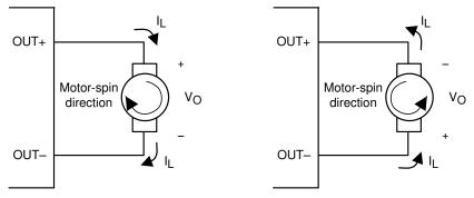
Figure 2-1. Motor Spin Direction in ERM Motors
