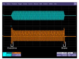
Figure 3-4. Typical Alert Effect With LRA in Closed-Loop
