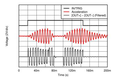
Figure 3-1. LRA Click With and Without Braking
