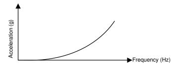
Figure 2-2. ERM Acceleration Versus Frequency Response
