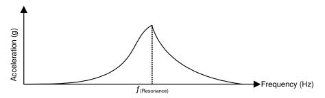
Figure 2-4. LRA Acceleration Versus Frequency Response
