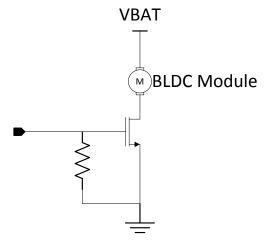
Figure 4-1. Circuit for Driving the BLDC
