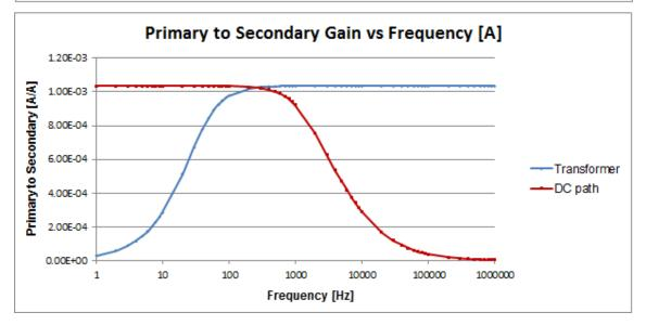
Figure 5. Closed Loop Gain vs. Frequency Response
