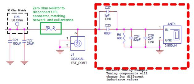
Figure 1. 0- $\Omega$  Resistor for Disconnecting the Matching Network
