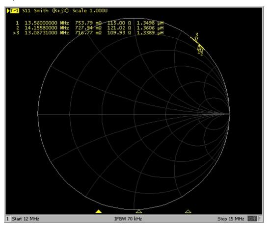
Figure 2. Smith Chart Capture From Network Analyzer
