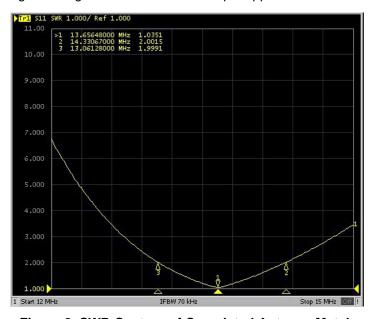
Figure 8. SWR Capture of Completed Antenna Match
