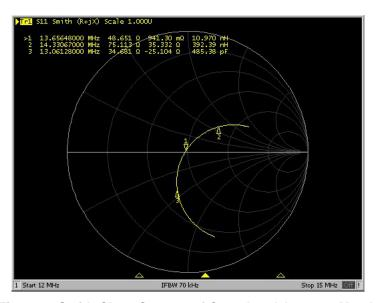
Figure 7. Smith Chart Capture of Completed Antenna Match
