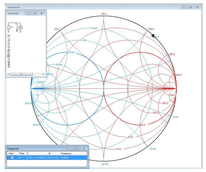
Figure 3. Complex Impedance Added to Smith Chart Simulator
