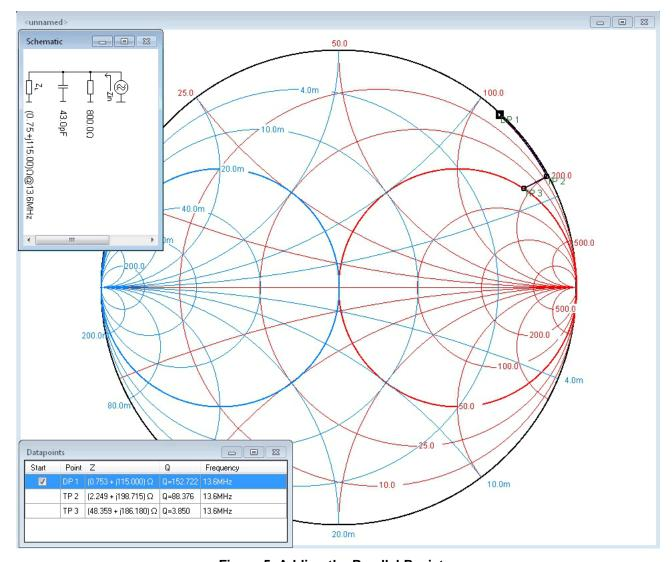
Figure 5. Adding the Parallel Resistor
