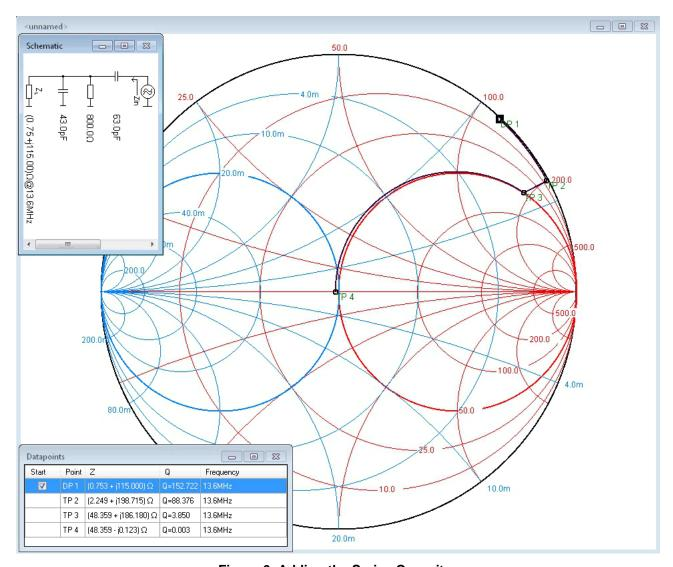
Figure 6. Adding the Series Capacitor
