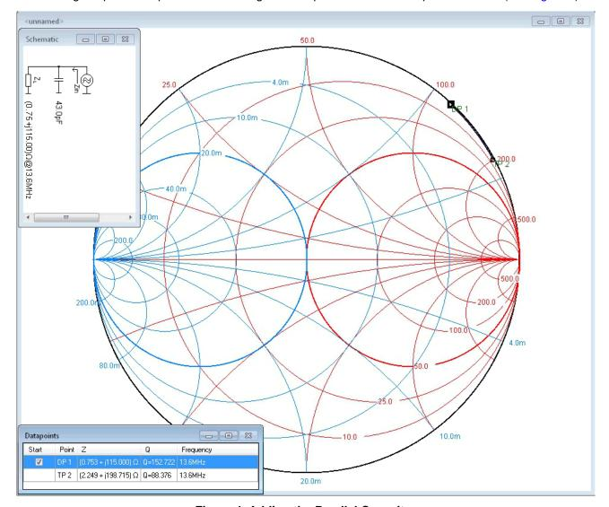
Figure 4. Adding the Parallel Capacitor
