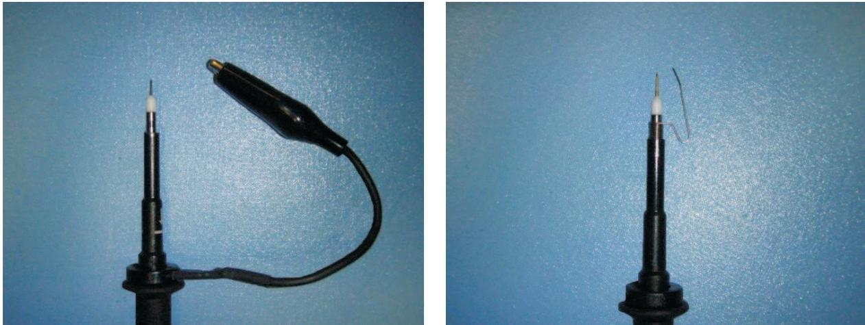
**Figure 8. Oscilloscope Probe Comparison: Typical 3-Inch Wire (Left) Versus Small Length Wire (Right)**
