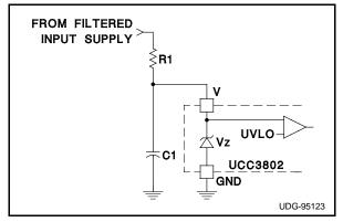
Figure 1. Off-line Current Source Power
