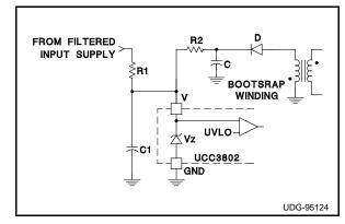
Figure 2. Adding a Bootstrap Supply
