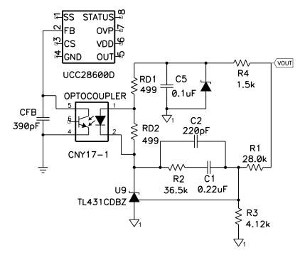
Figure 8. Typical Loop Compensation for the UCC28600
