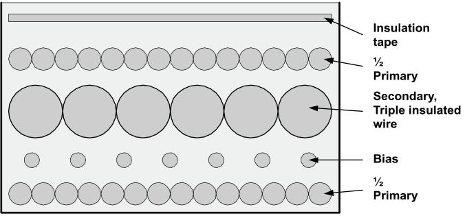
Figure 4. Example of a Recommended Transformer Design.
