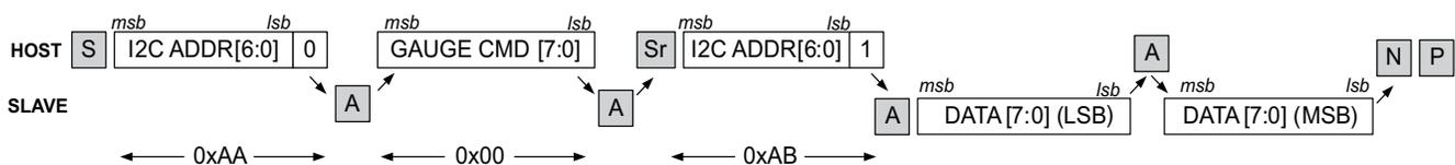
Figure 3. I<sup>2</sup>C Read Subcommand Sequence
