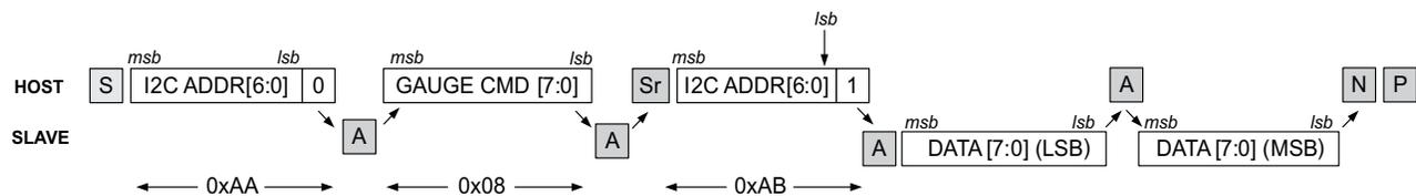
**Figure 1. Simple I<sup>2</sup>C Command Transaction Sequence**
