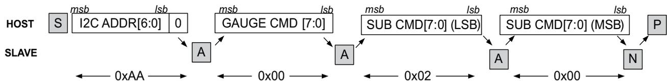
Figure 2. I<sup>2</sup>C Subcommand Initiation Sequence
