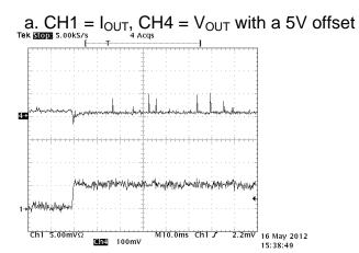
Figure 11, 0.1 to 0.6A load step
