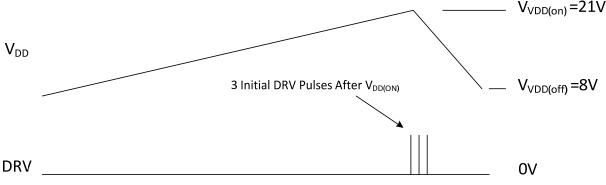
Figure 2, VDD and DRV at Startup with Fault
