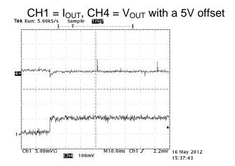
Figure 9, 0.1 to 0.6A load step
