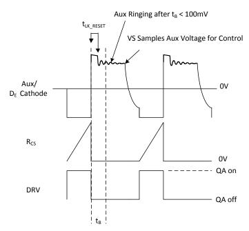
Figure 4, Auxiliary Winding VS Blanking
