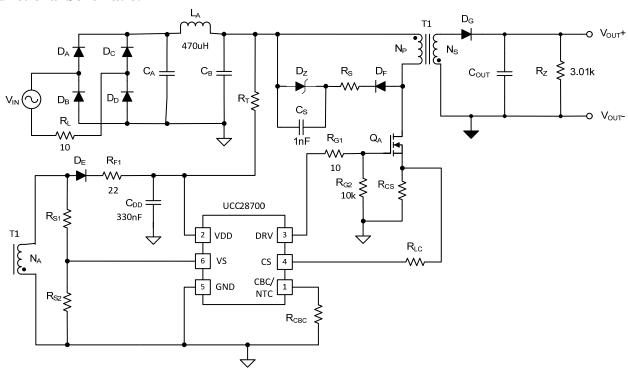
Figure 1, UCC28700 5W Offline Flyback Functional Schematic
