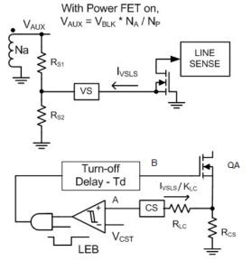
Figure 5, Peak Current Limit Comparator
