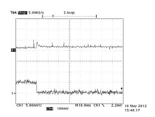
Figure 10, 0.6 to 0.1A load step
