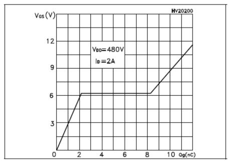
Figure 3, Gate Charge vs  $V_{\rm gs}$
