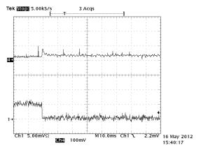
Figure 12, 0.6 to 0.1A load step
