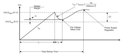
Figure 5. Timing Diagram of Startup Sequence in UCC28722
