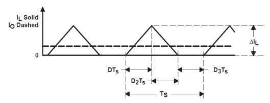
Figure 6. Discontinuous Current Waveform in UCC28722
