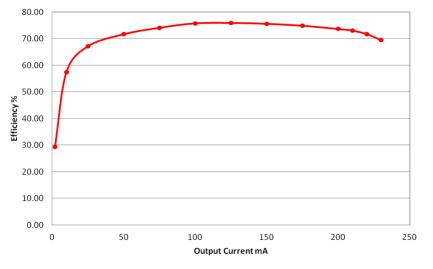
Figure 13. Efficiency vs O/p Load Current at 325 VDC
