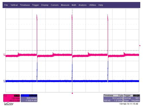
Figure 17. SW node Waveform and Collector Current at Vin = 275 VAC, Full Load
