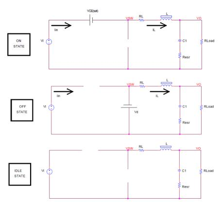
Figure 3. Buck Power Stages in Discontinuous Mode
