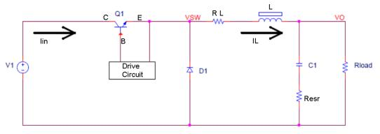
Figure 2. Buck Power Stage Schematic
