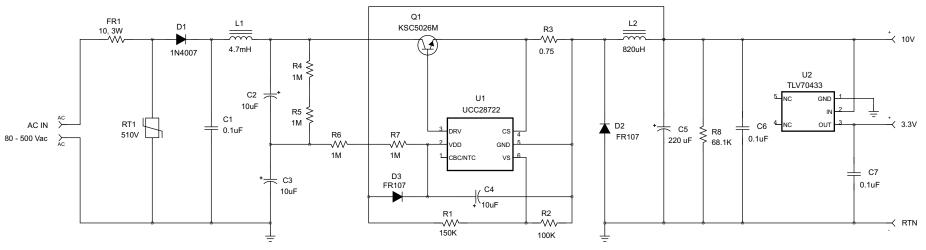
Figure 7. Complete Schematic of the PMP7668 Non-Isolated Buck Converter
