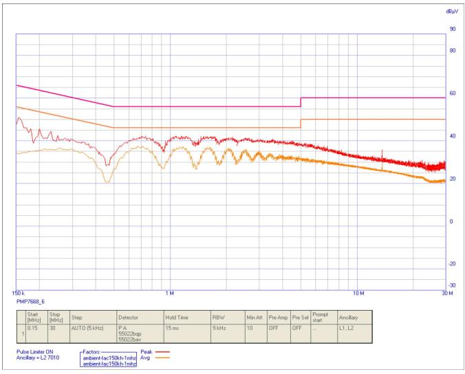
Figure 24. Conducted Emissions as per EN55022 Class B
