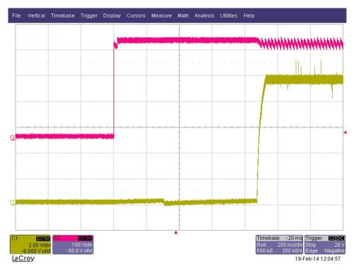
Figure 22. Vout Turn On Waveform at Vin = 275 VAC, Full Load
