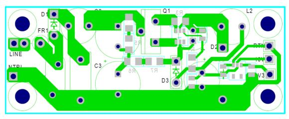
Figure 10. PCB Composite Layout
