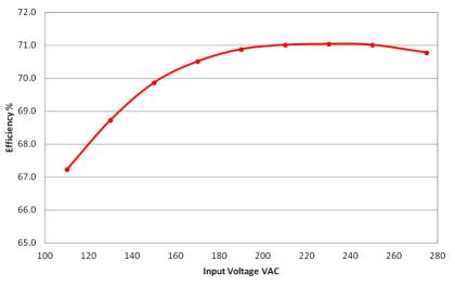
Figure 11. Efficiency vs AC I/p Voltage (110 V-275 V)
