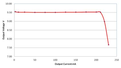
Figure 14. O/p Voltage Variation vs O/p Load Current at 325 VDC
