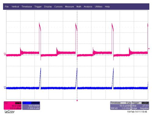
Figure 15. SW Node Waveform and Collector Current at Vin = 110 VAC, Full Load
