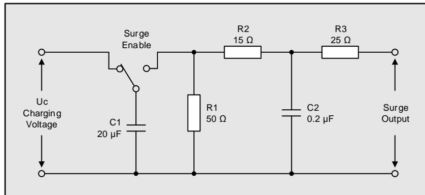
**Figure 1. ITU-T K.44 Impulse Generator as Defined in Figure N.1 of IEC 60950-1 Standard**
