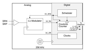
Figure 9. 16-Bit Delta Sigma Coulomb Counter
