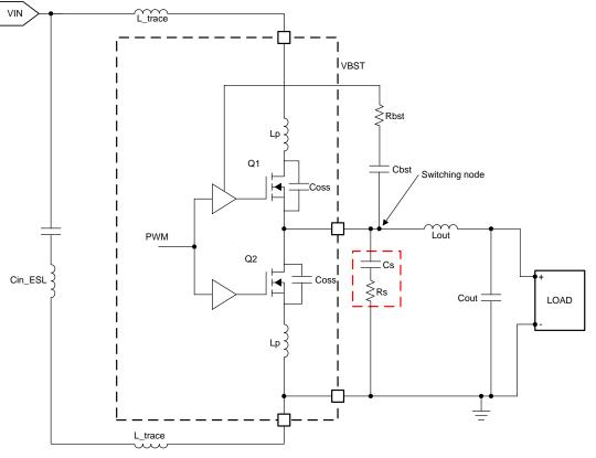
Figure 4. RC Snubber Added Circuit With Parasitic Components
