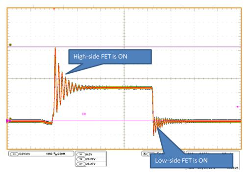
Figure 6. Switching Ringing Waveform Rising and Falling Edges
