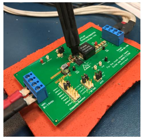
Figure 2. Probing Using 1-GHz Differential Probe
