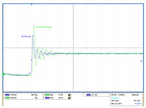
Figure 3. Typical Switching Ringing Waveform of TPS53355
