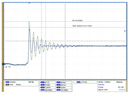
Figure 9. Switch Node Ringing Waveforms at 30-A Load (Blue: With Snubber 2.2nF + 1.47Ω, Green: No Snubber)
