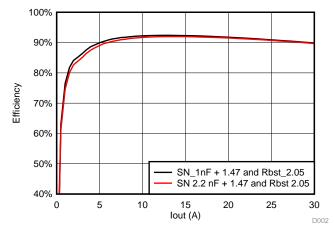
Figure 13. Efficiency Comparison When Snubber Capacitance Cs Changes
