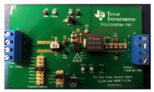
Figure 5. TPS53355EVM-743 RC Snubber Placements
