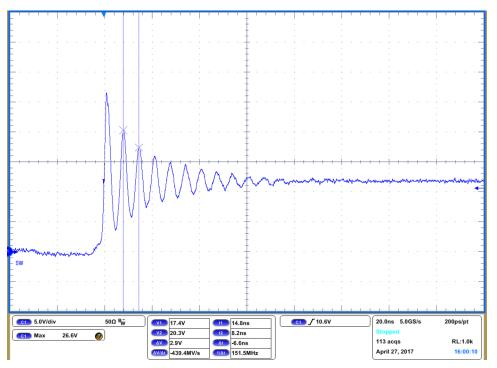
Figure 7. Un-snubber Switching Node Ringing Waveform
