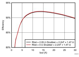
Figure 12. Boot Resistor Effects on Efficiency
