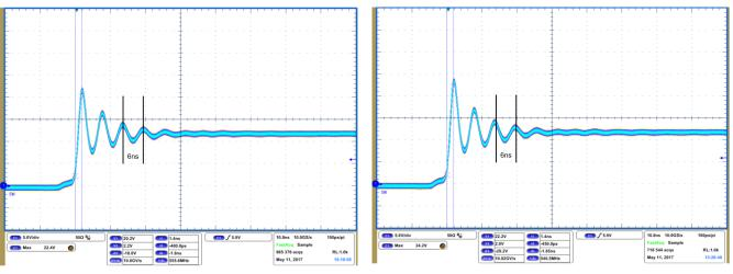
Figure 10. Rbst 2.05  $\Omega$  + 0.1  $\mu\text{F}$  and 1.47  $\Omega$  + 2.2 nF Snubber
