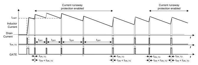
Figure 2. Current Runaway Protection Extends torFF Cycle-By-Cycle to Reduce Inductor Current
