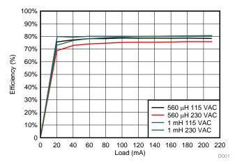
Figure 3. Efficiency Comparison for UCC28881EVM with 560 uH Saturating and 1 mh Standard Inductor
