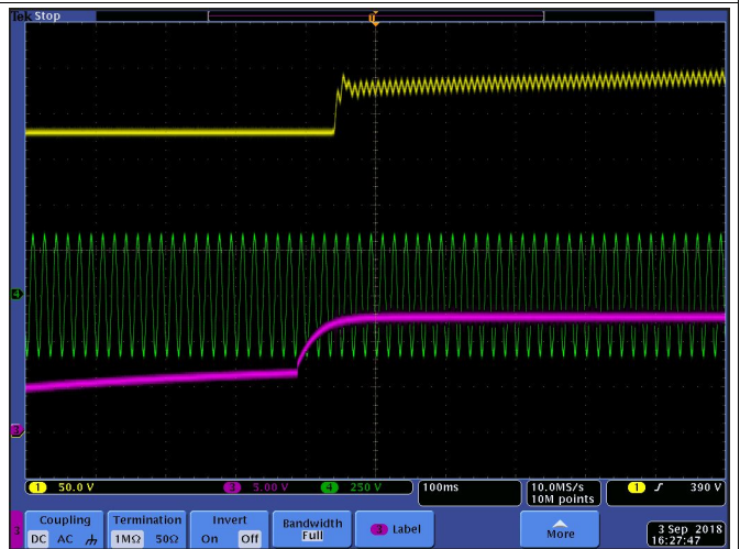
Figure 14. 230 V inac at FL
