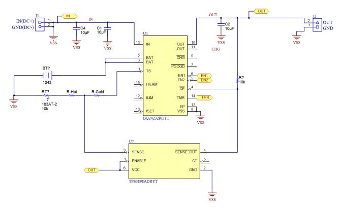
Figure 2. External Voltage Supervisor Solution
