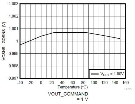
Figure 2. Output Voltage Versus Junction Temperature
