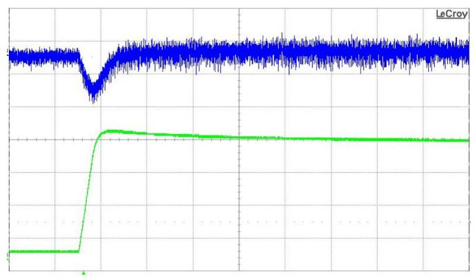
Figure 4. Load Transient with TPS546D24A and Internal Voltage Divider
