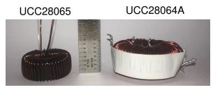
Figure 11. Boost Inductor Comparison
