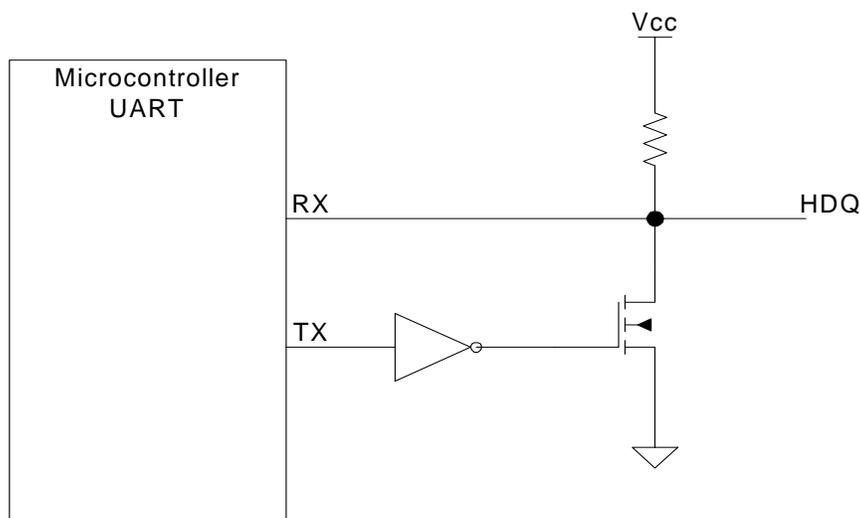
HDQ Communication Circuit For UART Without Open Drain Outputs
