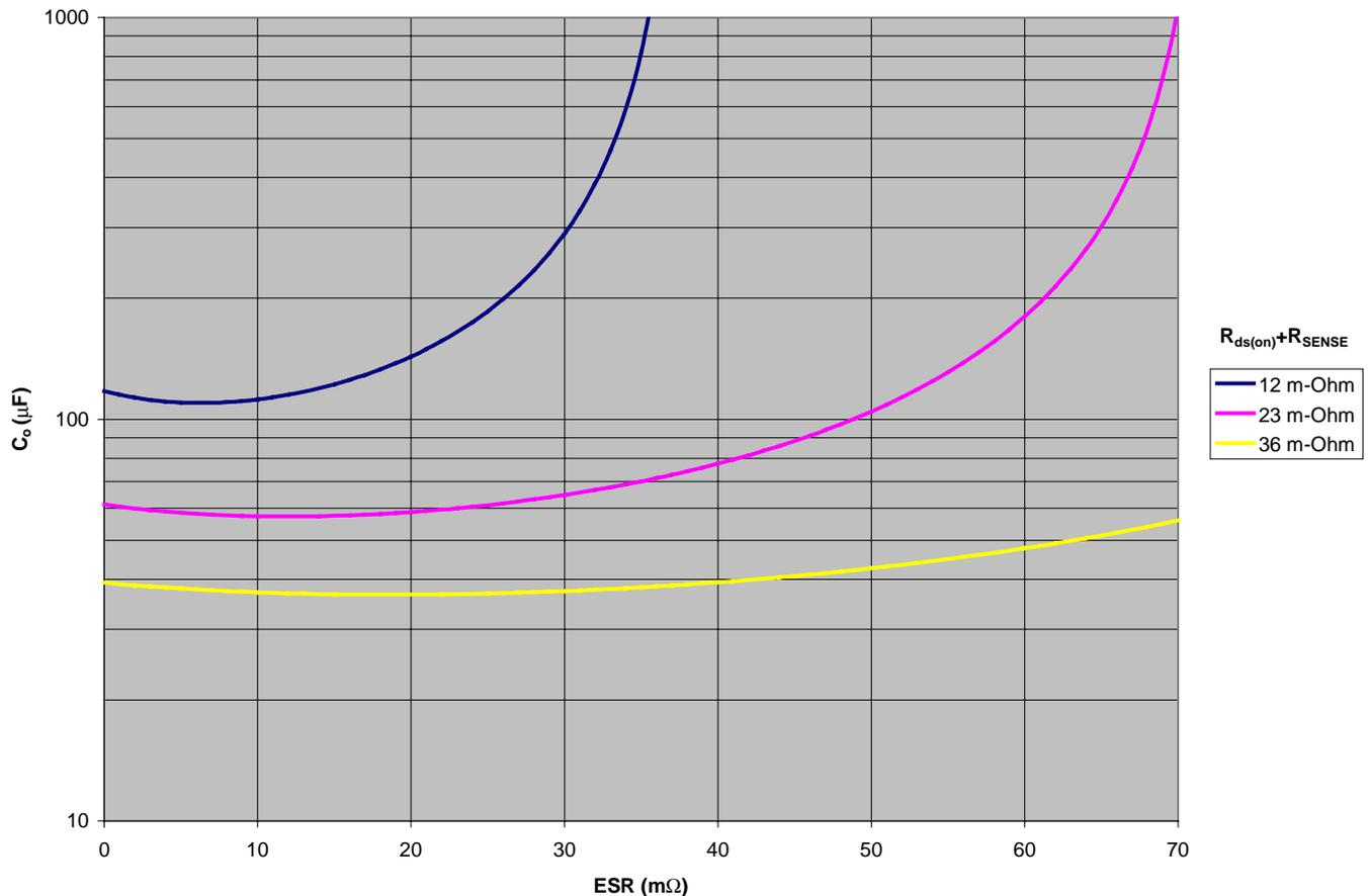
**Figure 4. Minimum Hold-Up Capacitance for V<sub>i</sub> = 3.3V and τ = 2μsec**
