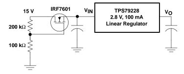
Figure 1. MOSFET Switch Used to Expand the Regulator's Input Voltage
