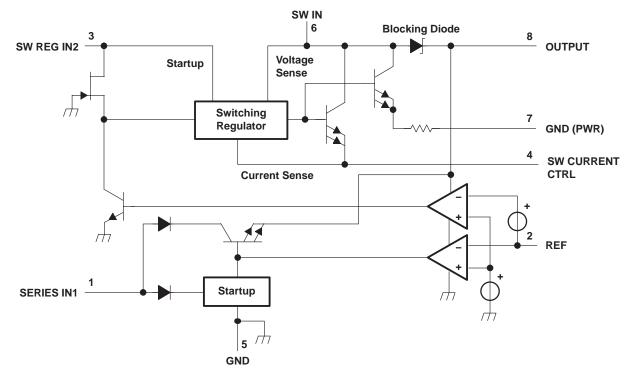
Figure 1. TL499A Block Diagram
