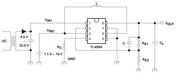
Figure 15. Battery-Backup Circuit
