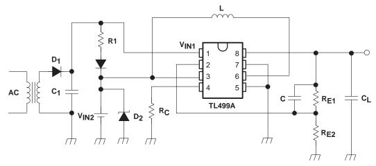
Figure 16. Charge-Protection Circuit
