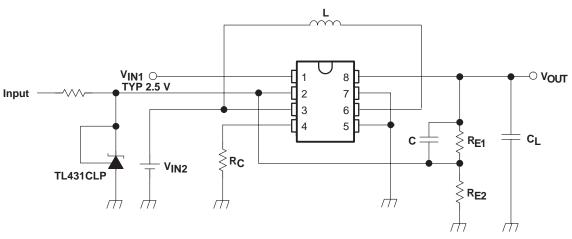
Figure 19. Switching-Inhibit Circuit Using Pin 2
