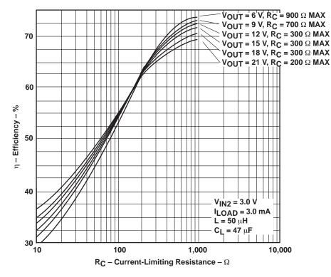
Figure 7. Step-Up Switching-Regulator Efficiency vs R<sub>C</sub>
