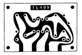
Figure 33. Recommended Board-Pattern Layout
