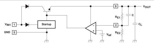
Figure 5. Internal Equivalent Circuit of Series Regulator
