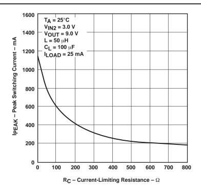
Figure 8. Peak Switching Current (IPEAK) vs Current-Limiting Resistance (R<sub>C</sub>), I<sub>OUT</sub> = 25 mA
