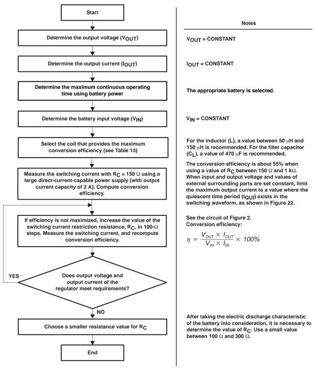
Figure 32. Switching-Regulator Design-Procedure Flowchart
