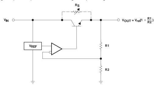
Figure 3. Basic Composition of Series Regulator
