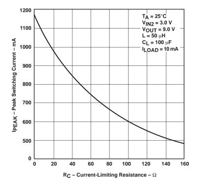
Figure 9. Peak Switching Current ( $I_{PEAK}$ ) vs Current-Limiting Resistance ( $R_C$ ),  $I_{OUT}$  = 10 mA
