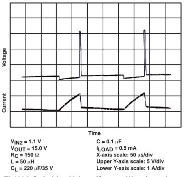
Figure 29. TL499A Switching Voltage/Current Waveform, ILOAD = 0.5 mA
