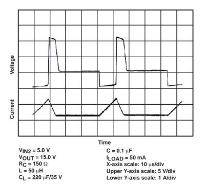
Figure 24. TL499A Switching Voltage/Current Waveform, ILOAD = 50 mA
