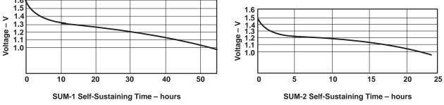
Figure 13. Discharge Characteristics of Dry-Cell Batteries
