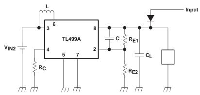
Figure 18. Switching-Inhibit Circuit Using Pin 8
