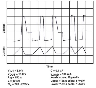
Figure 26. TL499A Switching Voltage/Current Waveform, ILOAD = 100 mA
