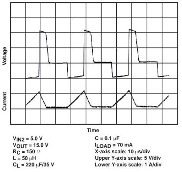
Figure 25. TL499A Switching Voltage/Current Waveform, ILOAD = 70 mA
