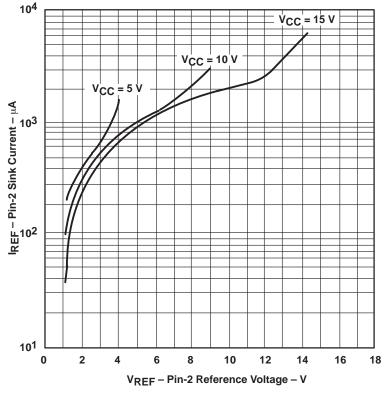
Figure 20. Pin-2 Sink Current vs Pin-2 Reference Voltage
