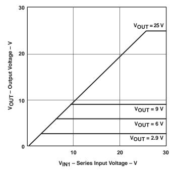
Figure 4. Series-Regulation Characteristic
