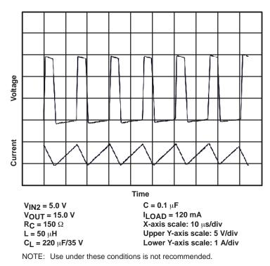
Figure 27. TL499A Switching Voltage/Current Waveform (Maximum Load)
