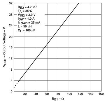
Figure 11. Output Voltage vs R<sub>E1</sub>
