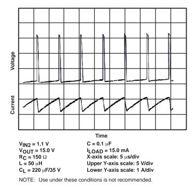
Figure 31. TL499A Switching Voltage/Current Waveform (Maximum Load)
