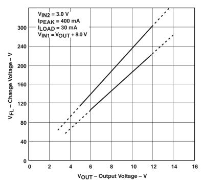
Figure 14. Change Voltage (V<sub>FL</sub>) vs Output Voltage
