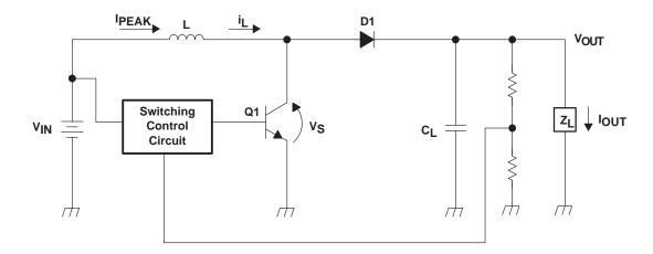
Figure 6. Basic Composition of Step-Up Switching Regulator
