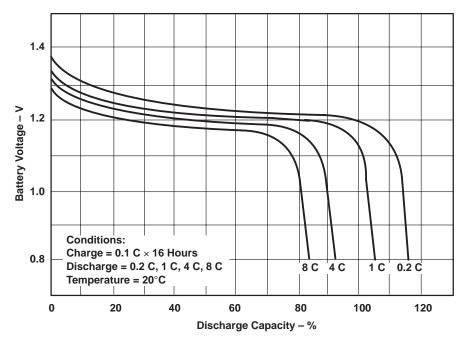
Figure 12. Discharge Characteristics of Nickel-Cadmium Batteries
