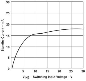
Figure 17. Standby-Current Characteristics
