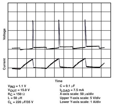
Figure 30. TL499A Switching Voltage/Current Waveform, ILOAD = 7.5 mA
